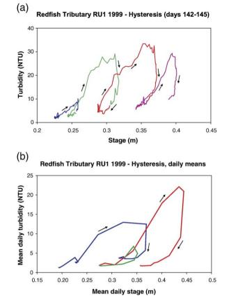
Fig. 9. Graphs showing hysteresis of turbidity. The data are from the turbidity and water level record shown in Fig. 7. (a) Four days of record (days 142–145) during a peak snowmelt period; data points are every 15 min. (b) Daily mean turbidity and water level for a 4-week period which includes most of the seasonal snowmelt runoff.
