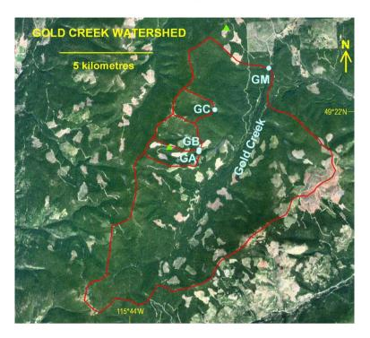
Fig. 3. Map of Gold Creek watershed, based on a satellite image. Round dots and labels indicate the four streamflow and sediment monitoring stations. GM is the site of the hydrometric station on Gold Creek; GA, GB, and GC are the detailed study tributaries. Triangles are climate stations.
