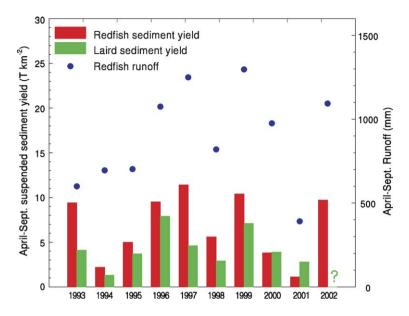
Fig. 10. April–September suspended sediment yields for Redfish and Laird Creeks, and runoff for Redfish Creek, for the 10-year period of record. The 2002 yield for Laird Creek is missing, as bedload movement interfered with the automatic pump sampler.
