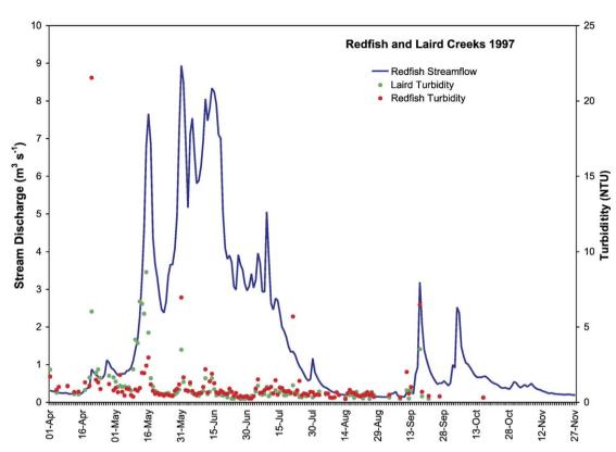
Fig. 6. Example of a hydrograph of mean daily discharge for Redfish Creek for one season, and turbidity samples for Redfish and Laird Creeks.
