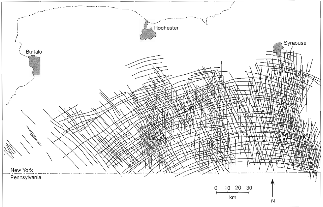
Figure 3.12 Map of joints in the Appalachian Plateau in New York state. The lines are constructed parallel to the dominant strike of joints measured in local outcrops throughout the area.
