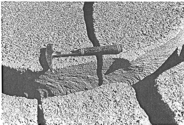
Figure 3.13 Plumose structure, or hackle plumes, in A mudstone, and B chalk.
