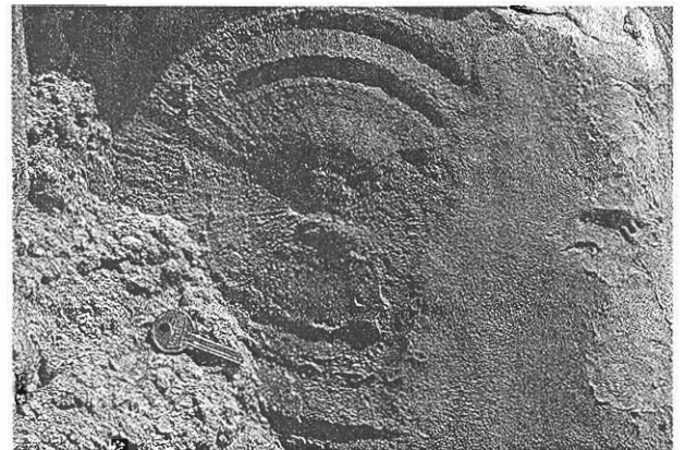
Figure 3.13 Plumose structure, or hackle plumes, in A mudstone, and B chalk.
