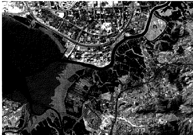
Figure 4.2.2.h Landsat 5,4,2 (RGB) false color composite image of the eastern end of Deep Bay with 30 m resolution.
