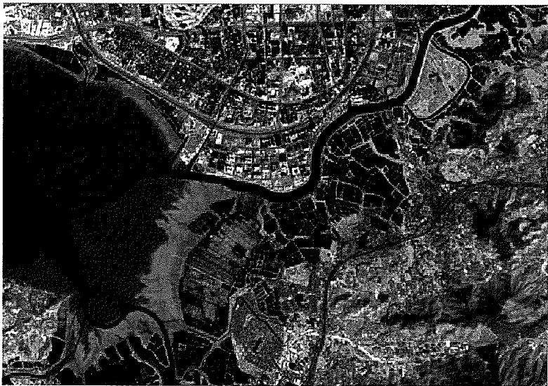
Figure 4.2.3.h Multiplicative merge of Landsat bands 5,4,2 (RGB) and the panchromatic band, with approximately 15m resolution.
