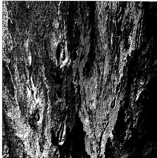
Figure 6.3.5.g TIMS false color composite of saturation-stretched data. Band 1 as blue, band 3 as green and band 5 as red.
