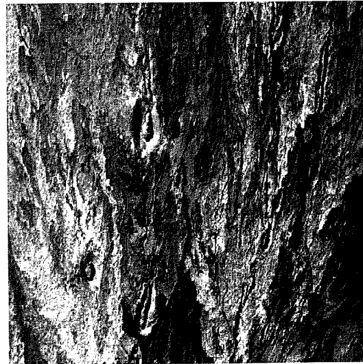
Figure 6.3.2.a TIMS false color composite. Band 1 (8.15 - 8.5 \mu\text{m} ) as blue, band 3 (9.0 - 9.3 \mu\text{m} ) as green and band 5 (10.3 - 11.1 \mu\text{m} ) as red.
