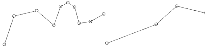
The original polyline is on the left. The polyline smoothed with Vertex Averaging (Average Rate = 3) is shown on the right.
