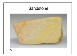
Sandstone • Composed of sand-size particles – Between 1/16 mm and 2 mm diameter – Particles may be individual mineral grains or rock fragments – Quartz most common type of grain
