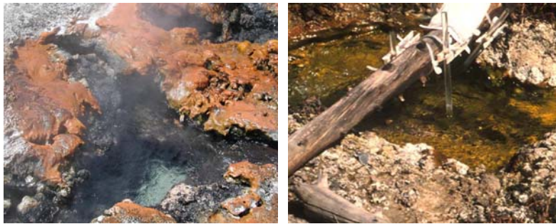
Figure 1 (left): Fairy Hot Spring at Yellowstone National Park. The bright orange surrounding the water is the mat system. Figure 2 (right): This is a picture of the experimental set up with the glass rods. The rods were placed so that they were in the water but not touching the floor of the run-off and had enough area above the water for splashing and mat formation to occur.
