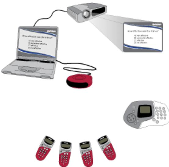
Qwizdom's **Response System** includes a host, which plugs into the instructor's laptop or desktop USB drive, teacher remote, and student remotes. The host transmits a radio frequency which allows communication with the instructor's computer, the teacher remote, and student remote. This RF IEEE standard system helps insure robust, conflict-free operation and supports up to 1,000 remotes at one time. The Qwizdom Participant Remote provides instant feedback to participants.
