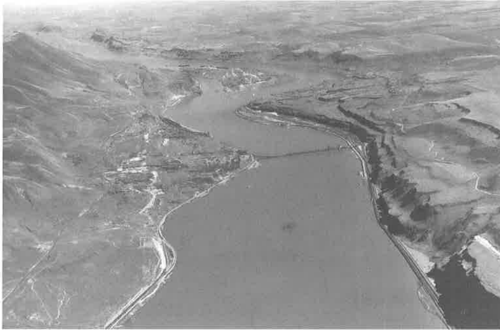
The Columbia Hills to the left are the up-thrown block of a large east-west reverse (compressional) fault. Looking east up the Columbia River, Wishram, Washington, is left center and the mouth of the Deschutes River is on the upper right. (Photo courtesy Oregon Department of Transportation)
