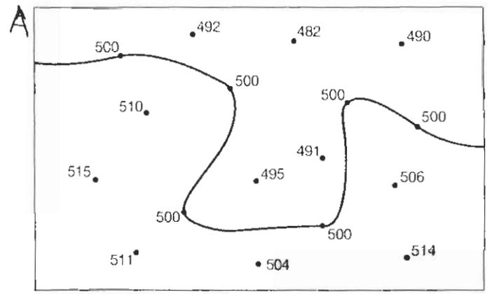
**FIGURE 8.11** Topographic map construction (elevations are in feet). Notice in map A that a 500-foot contour line has been drawn through all the points that have an elevation of 500 feet above mean sea level. Can you finish contouring both maps using a contour interval of 10 feet?
