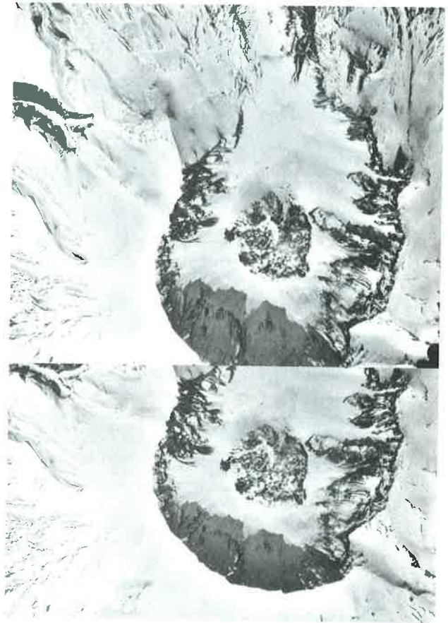
FIGURE 5.4(B) Vertical aerial stereographic photos of Mount St. Helens after the May 18, 1980, eruption (USGS).
