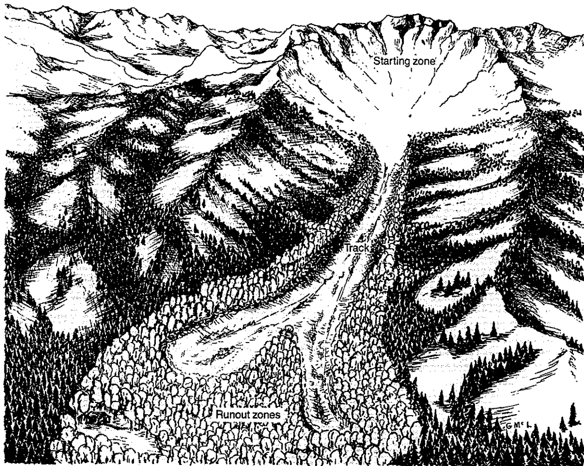
FIGURE 8.25 Large avalanche path showing various features. The smaller runout zone, reached more frequently, is cut through the aspen forest. The larger zone is reached much less frequently, is revegetated by aspen, and must be considered in planning any development (Mears, 1976; after Salm, 1975).
