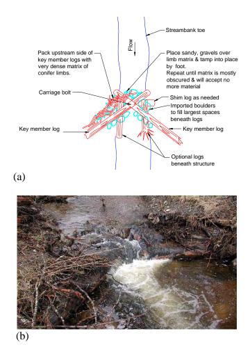
**Large Wood and Log Jams Figure 17**. A V-shaped log sill created with two crossed logs: (a) concept sketch showing small wood on upstream side of log to retain streambed sediment; (b) photo of crossed log structure (unidentified creek near Pysht River, Clallam County, Washington).
