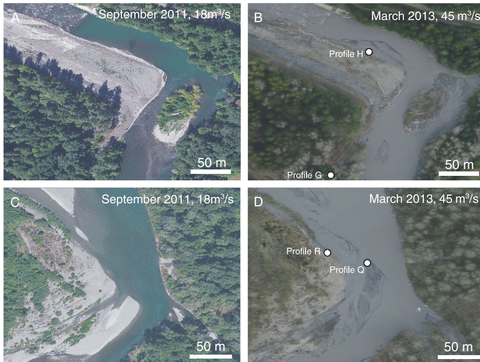
Figure 3. Orthorectified aerial images showing contrast between pre- and post-dam-removal channel configuration and fluvial sediment. (A) and (B) show a location 2 km downstream of the Elwha Dam site (15.7 km downstream of the Glines Canyon Dam site) in September 2011 and March 2013, respectively; engineered riffle at the top of these images is part of the Elwha Surface Water Intake facility diverting water toward a fish hatchery and municipal water-treatment plant. (C) and (D) show a location 7.2 km downstream of the Elwha Dam site (20.9 km downstream of the Glines Canyon Dam site) in September 2011 and March 2013, respectively. Locations of sedimentary profiles sampled for this study are shown in (B) and (D). Differences between (A) and (B) and between (C) and (D) include the appearance of new sediment that is finer than the pre-dam-removal cobble bed, and formation of new mid-channel bars. The post-dam-removal fine sediment also has a dark grey colour distinct from that of the older cobble bed. Discharge in the September 2011 images (A) and (C) is 18\text{ m}^3/\text{s} ; discharge in the March 2011 images is 45\text{ m}^3/\text{s} . 2011 images courtesy of the U.S. Department of Agriculture, National Aerial Imaging Program. 2013 images by A.C. Ritchie. This figure is available in colour online at wileyonlinelibrary.com/journal/trra
