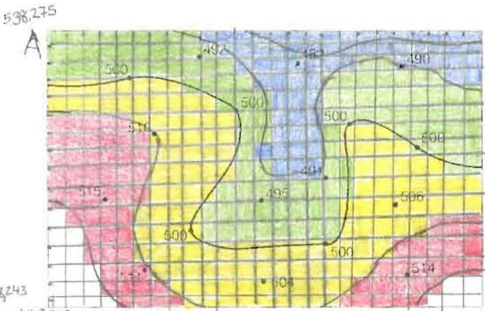
**FIGURE 8.11** Topographic map construction (elevations are in feet) Notice in map A that a 500-foot contour line has been drawn through all the points that have an elevation of 500 feet above mean sea level. Can you finish contouring both maps using a contour interval of 10 feet?
