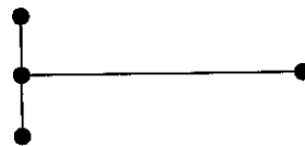
Correct topology—the horizontal line intersects the vertical one, creating three lines.
