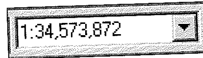
Fig. 2.12. The scale box in ArcMap shows the current scale of the map on the screen.
